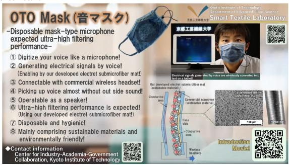
Figure 1. Overview diagram of "OTO Mask"
